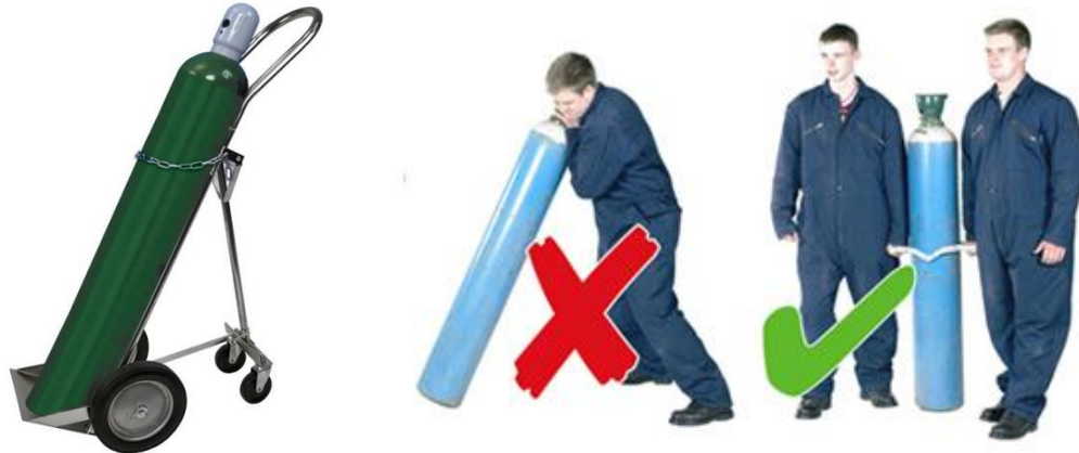
Fig: Proper method to transport cylinders. (left) using tank carts (b) two people holding a cylinder upright.
