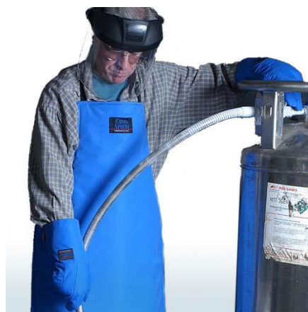
Fig: The correct usage with proper protective equipment + use of both hands to hold the tank and tube.
