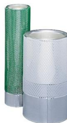
Fig: (left) Liquid dewar flasks of different sizes. (right) laboratory liquid dewar flask
