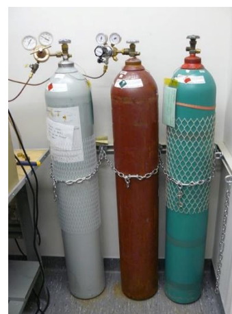
Fig: (left) How to store cylinders in long term. (right) correct way of storing cylinders during use.
