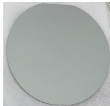
Liquid phase crystallized Ge-on-Si 2"-wafer.
