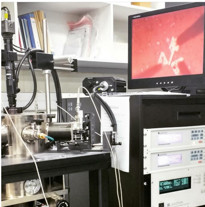
Figure 2: Performing Temperature dependent measurements in Helium Probestation (in MNCF) to understand the transport mechanism of the transistors.
