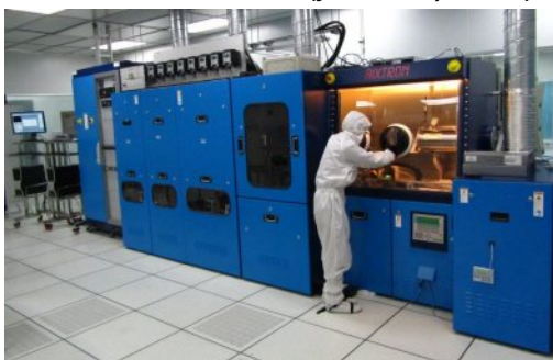
The GaN reactor (funded by SSPL/DRDO) in the CeNSE clean room (funded by Deity).
