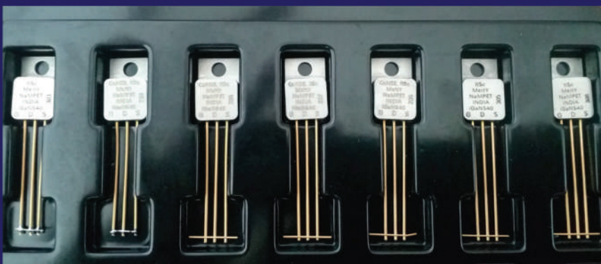
Packaged power transistors that can carry 5Amp of current, ready to be shipped to CDAC, Trivandrum for making DC-DC converters
